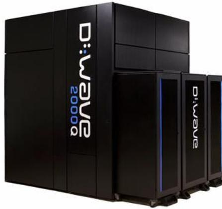
External disturbances cause quantum computers to lose their quantum coherence, so they must be completely isolated in an enclosed case at an extremely low temperature. They also must be isolated from Earth's magnetic field. Quantum computers can be used for cryptography, search problems, simulation of quantum systems, quantum annealing and adiabatic optimization, machine learning, computational biology, and computer-aided drug design and generative chemistry.
